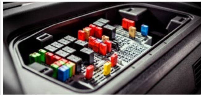
In-cab electrical panel is protected from the elements and conveniently located under spill-resistant dash panel
