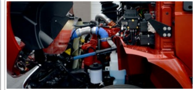
Key fluid reservoirs are translucent for quick inspection and many of the caps are tethered, saving time and frustration from dropped or lost caps
