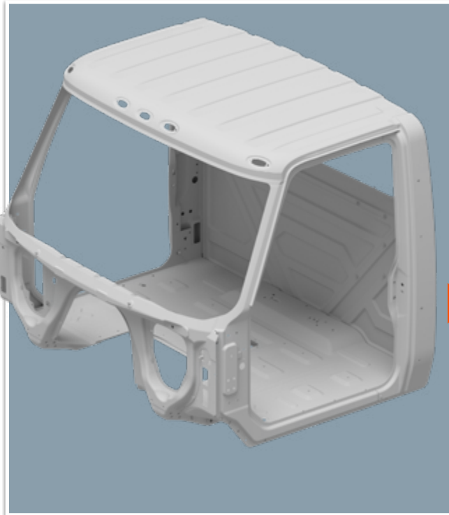
One continuous piece of steel surrounds the entire door frame for superior structural integrity, durability and sealing
